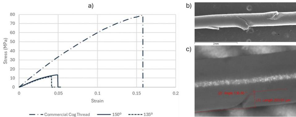
Figure 2 – a) Stress-strain values obtained from uniaxial tensile tests on both commercial and printed cog threads. b) SEM image of the commercial cog thread. c) Microscope image of the printed cog thread.
