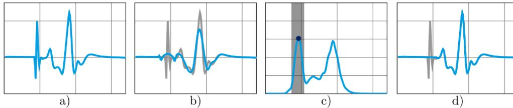
Figure 1 –Filtering process: a) raw data with both the artifact and the M-wave present; b) Savitzky-Golay Filter applied to the raw data; c) Residue between filtered and raw data is full-wave rectified, low-pass filtered and the first peak of the M-shape is used to create the exclusion region; d) the artifact is removed from the raw data and the final signal is interpolated to get an artifact-free M-wave.
