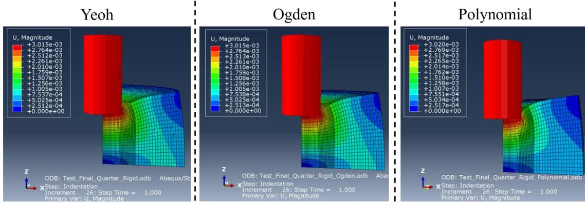
Figure 2 – Displacement results for each hyperelastic model tested: Left – Yeoh model; Middle – Ogden model; Right – Polynomial model (N=2)
