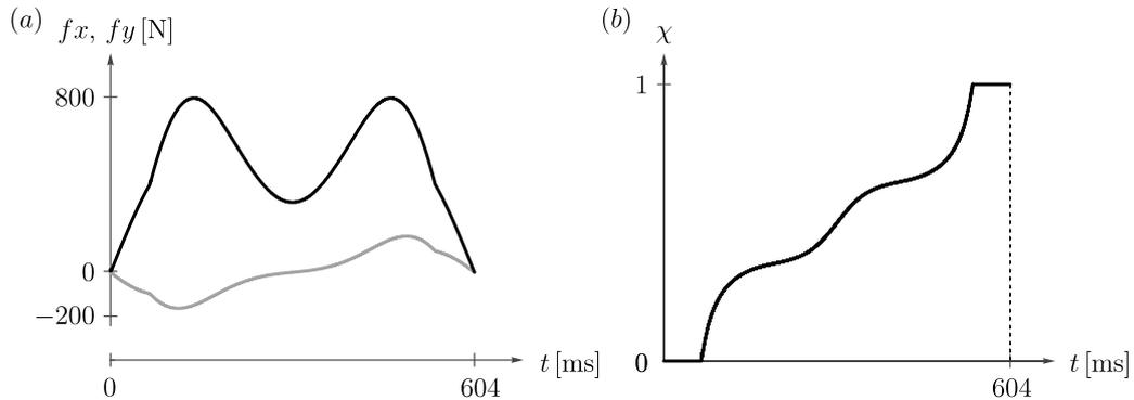
Figure 2. Stable periodic solution, with  $m = 75 \text{ kg}$ ,  $\varphi_c(0) = \varphi_b(0) = 1 \text{ m}$ ,  $k = 9 \times 10^3 \text{ [N/m]}$  and  $\ell_p = 15 \text{ cm}$ . (a) Force profile along  $x$  (gray) and  $y$  (black). (b) Pressure center, from calcaneus ( $\chi = 0$ ) to ball ( $\chi = 1$ ).
