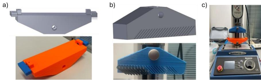
Figure 1 - a) Tool of fixation and rotation of the PCL fibres. b) Cutting tool. c) Multitest 2.5-dV machine equipped with the fixation, rotation, and cutting tools.
