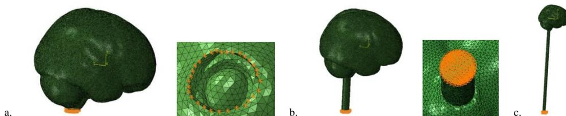
Figure 1 –Illustration of the applied boundary conditions: a. Skull BC; b. Neck BC; and c. Spine BC.
