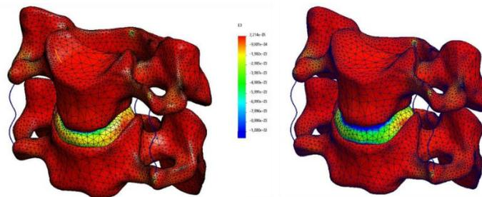
Figure 2 – Strain distribution in native model and degenerated.
