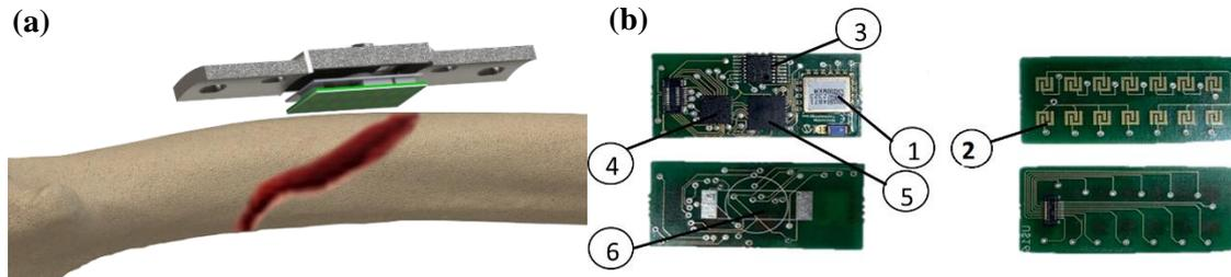
Figure 1- (a) Fractured bone with the new bioelectronic implant; (b) Electronic components: 1- Bluetooth module; 2- Capacitive matrix; 3-Analog-Digital convertor; 4-Multiplexer; 5- PIC16LF1847; 6- Battery.
