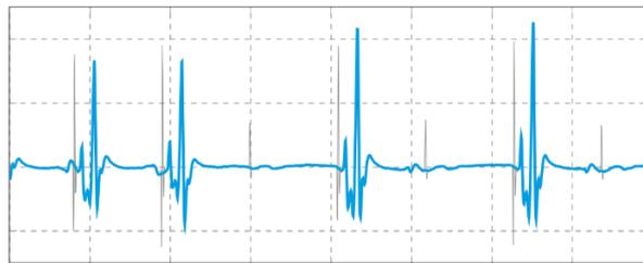
Figure 2 –Filtering of an EMG signal contaminated with artifacts from a 20Hz stimulation. One can see the raw signal (in grey) overlapped by the filtered signal (blue)
