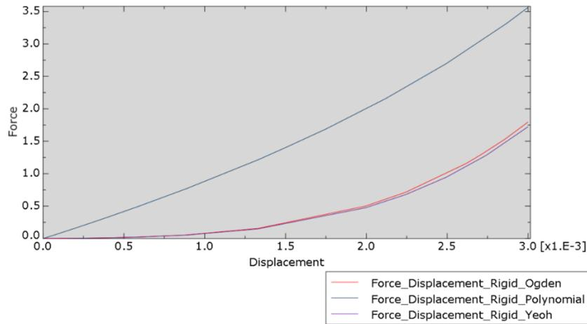
Figure 3 –Force (N) vs. Displacement (m) results for each model used
