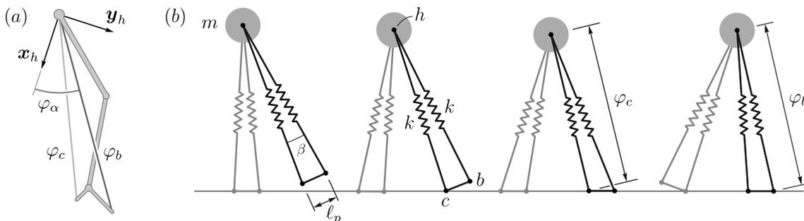
Figure 1. (a) Triangular leg coordinates. The  $\varphi_\alpha$  coordinate is measured with respect to the torso orientation, which is not illustrated. (b) Triangular spring-mass model. Illustrated from simulation (Fig. 2).
