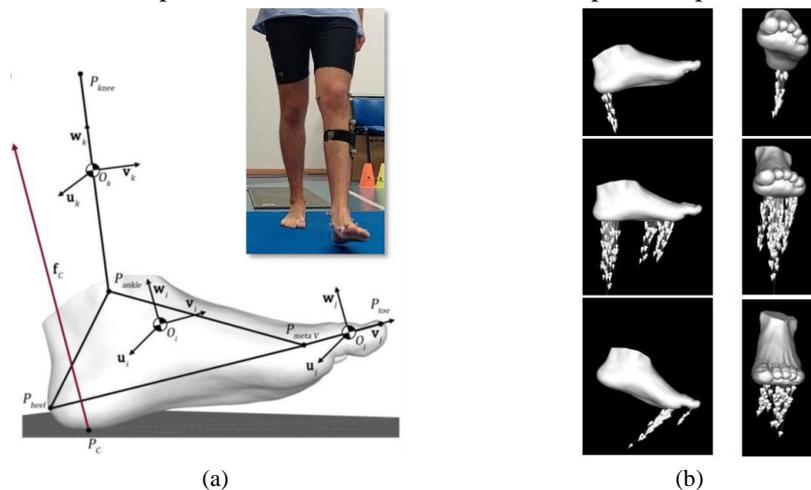
Figure 1 – (a) Experimental protocol and multibody model; (b) FEM model w/ contact forces and application points.
