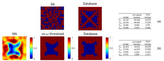
Figure 3 - Unit cell solutions using a surrogate model for homogenization and (a) a genetic algorithm (b) a neural network for unit cell design
