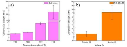
Figure 3. Compressive strength of a) bulk ceramics sintered at different temperatures and b) TPMS structures sintered at 1400°C.
