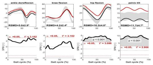
Figure 1. Pelvic and lower limb joint angles computed with the marker-based (red) and markerless (black) systems, and correspondent paired t-test performed with SPM1D.
