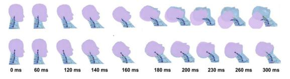
Figure 2 – Kinematics: ENM-2D (initial on top and final on bottom) and TNO-HBM (reference). After the optimization, both models' frames overlap, and ENM-2D is displayed in the front.
