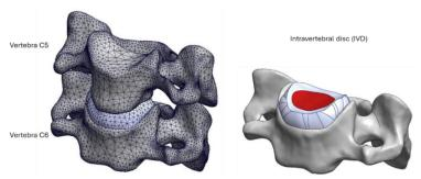
Figure 1 –Computational model of C5 and C6 cervical vertebra.
