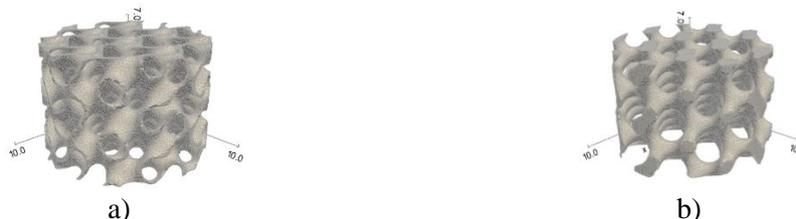
Figure 1 – Different lattices of a Gyroid with 80% porosity and 3mm cell size: a) Sheet, b) Network.
