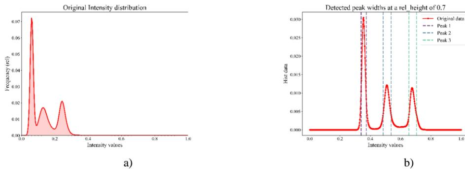
Figure 2 – a) Original gray level histogram, b) Segmented histogram and peaks, and thresholds detected.
