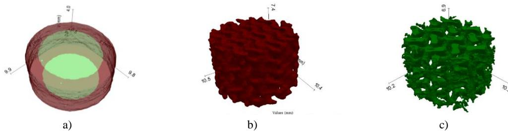
Figure 3 – Segmentation outputs: a) for the hollow cylinder (red) filled with powder (green); b) produced scaffold, c) trapped unsintered powder inside its pores.
